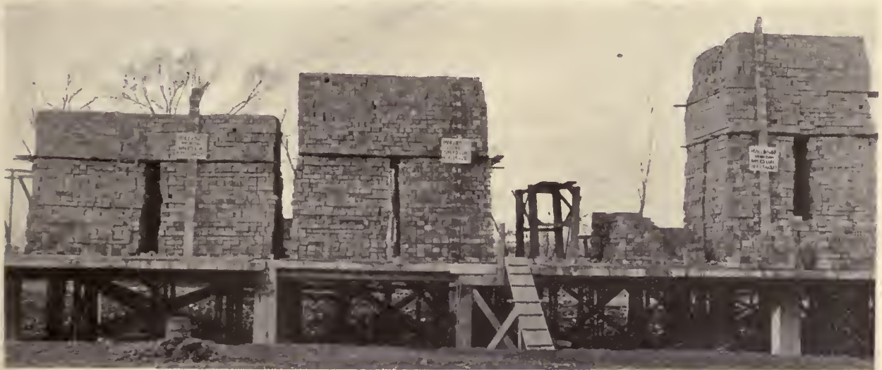
LOADING OF PANELS H, J AND K AT THE TIME OF THE NOVEMBER TEST Panels are lettered right to left
